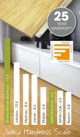
The higher the number, the harder the surface. All measurements are shown in kilonewtons (kN)
